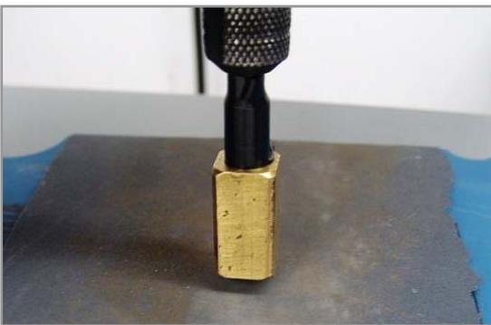
This is where patience comes in. Only put the seat and paper in contact with each other for a few moments. Then shut the tool off and check the seat. If the groove is gone, you are done. If not give it another turn on the paper. It usually takes me 8-10 turns on the paper to get a seat completely smooth.
