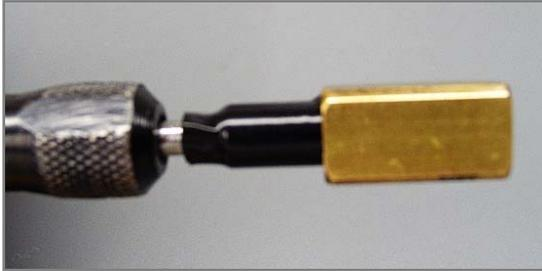
If you are doing a *Mistral* HP seat you will need to put a couple of turns of tape around the mandrel to make the seat fit tightly inside it.
