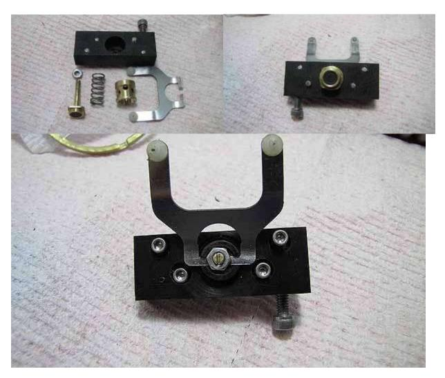
The next feature of the second stage is it's adjustable venturi. Again, calculating the needed flow and orifice sizes is not my strong suit so I opted for a more mechanical approach, an adjustable flow, besides; I wanted a way to vary the venturi response. I prefer a stronger venturi but others don't so I made a simple way to control the flow. The screw in the side of the body is turned to control the flow.
